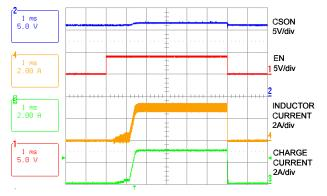
FIGURE 10. CHARGE ENABLE AND SHUTDOWN
