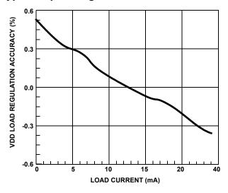
FIGURE 4. VDD LOAD REGULATION
