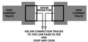
FIGURE 25. CURRENT SENSE RESISTOR LAYOUT
