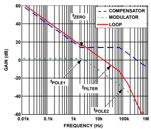
FIGURE 20. CHARGE CURRENT LOOP BODE PLOTS
