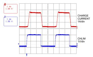
FIGURE 16. TRICKLE TO FULL-SCALE CHARGING
