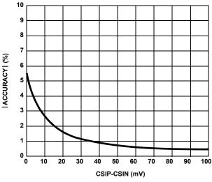
FIGURE 6. ACCURACY vs AC ADAPTER CURRENT
