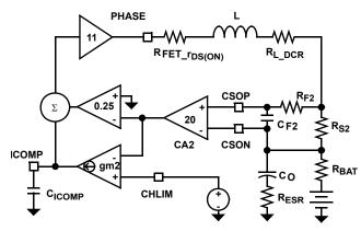
FIGURE 19. CHARGE CURRENT LIMIT LOOP
