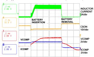
FIGURE 11. BATTERY INSERTION AND REMOVAL
