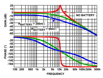
FIGURE 23. FREQUENCY RESPONSE OF THE LC OUTPUT FILTER
