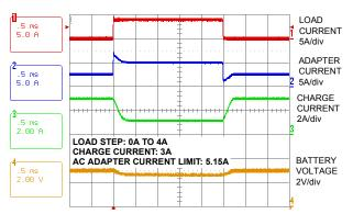
FIGURE 9. LOAD TRANSIENT RESPONSE
