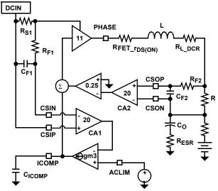
FIGURE 21. ADAPTER CURRENT LIMIT LOOP
