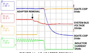
FIGURE 14. AC ADAPTER REMOVAL
