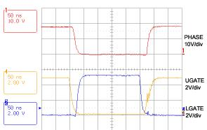
FIGURE 13. SWITCHING WAVEFORMS IN CC MODE
