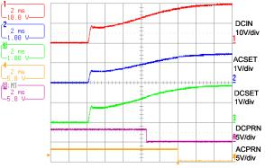
FIGURE 8. AC AND DC ADAPTER DETECTION
