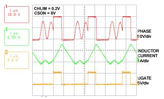
FIGURE 12. SWITCHING WAVEFORMS AT DIODE EMULATION
