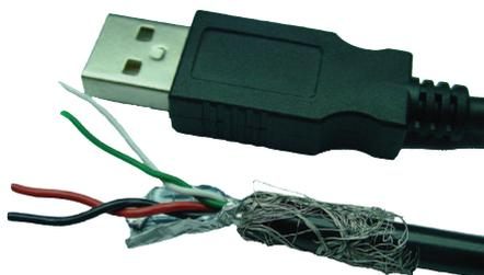
General construction: this is a USB-2.0 cable containing one 28 AWG 90Ω characteristic impedance data pair, two 24 AWG power conductors, overall SFTP shields (SFTP = double shielding, braid and foiled), jacketed in black UV resistant Polyurethane HFFR\*. Designed for fixed or portable applications in industrial and harsh environments.
