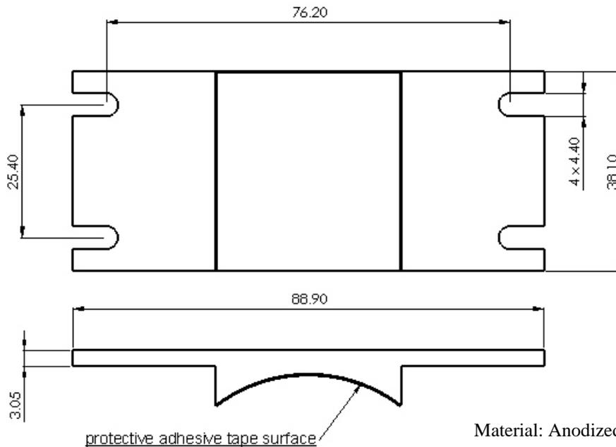
**For models with connectors SMA, QMA, SMA 2.9, Din 1.6/5.6**
