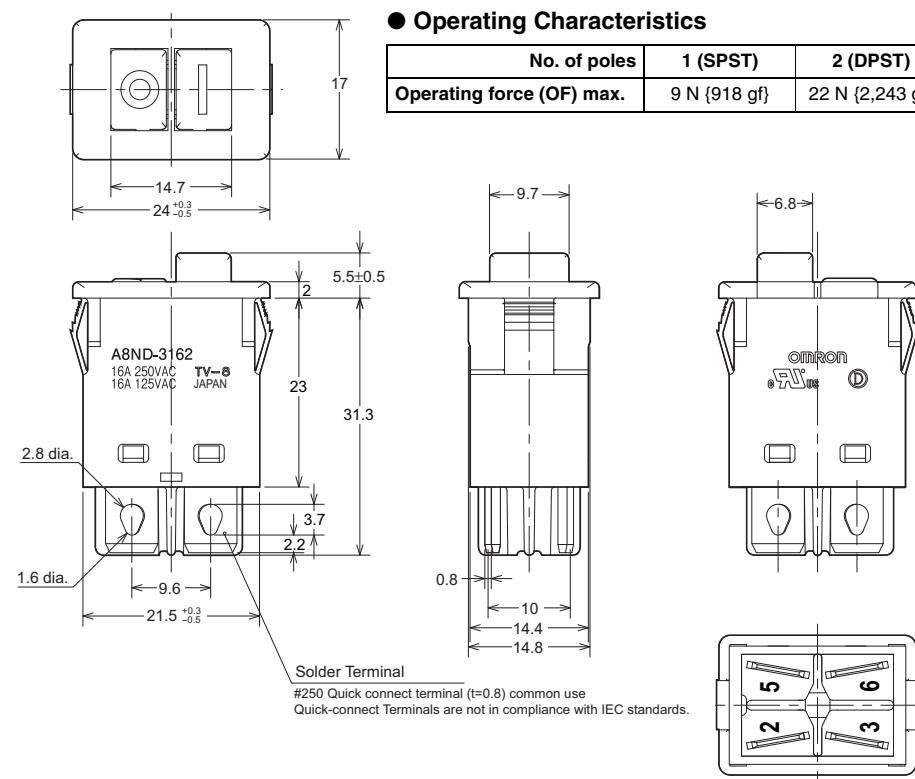
**Note:** Unless otherwise specified, a tolerance of  $\pm 0.3$  mm applies to all dimensions.
