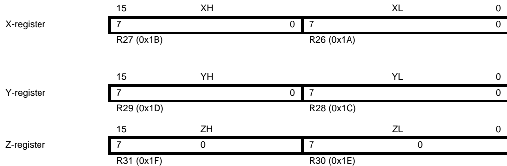
Figure 4-3. The X-, Y-, and Z-registers
