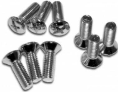
The screw provides a standard 0.625" rack screws length with 10-32 threads. The screw itself features a slotted and phillips, oval head and has a nickel plate finish.
