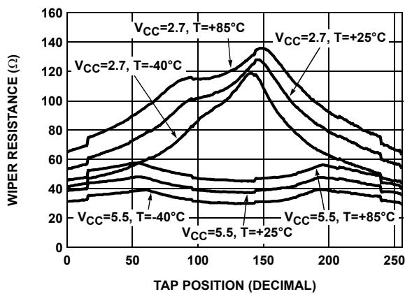
**FIGURE 1. WIPER RESISTANCE vs TAP POSITION**
