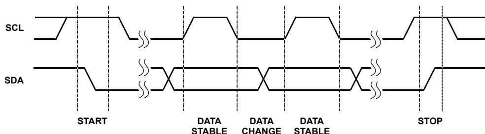
FIGURE 9. VALID DATA CHANGES, START, AND STOP CONDITIONS
