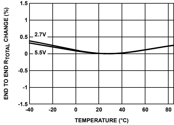
**FIGURE 5. END TO END  $R_{TOTAL}$  % CHANGE vs TEMPERATURE**
