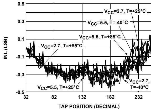
**FIGURE 4. INL vs TAP POSITION FOR  $50\text{k}\Omega$  (U)**
