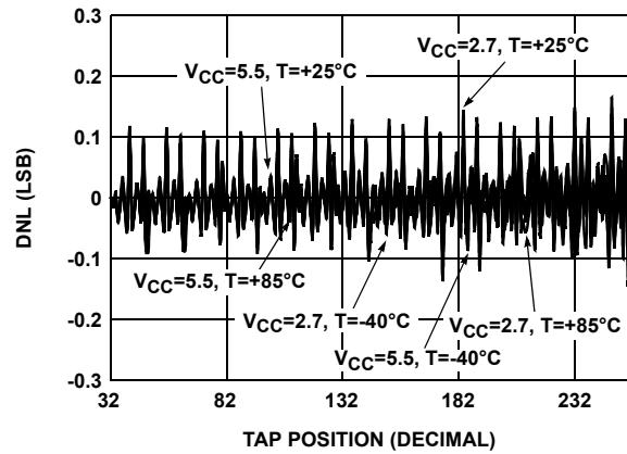
**FIGURE 3. DNL vs TAP POSITION FOR  $50\text{k}\Omega$  (U)**
