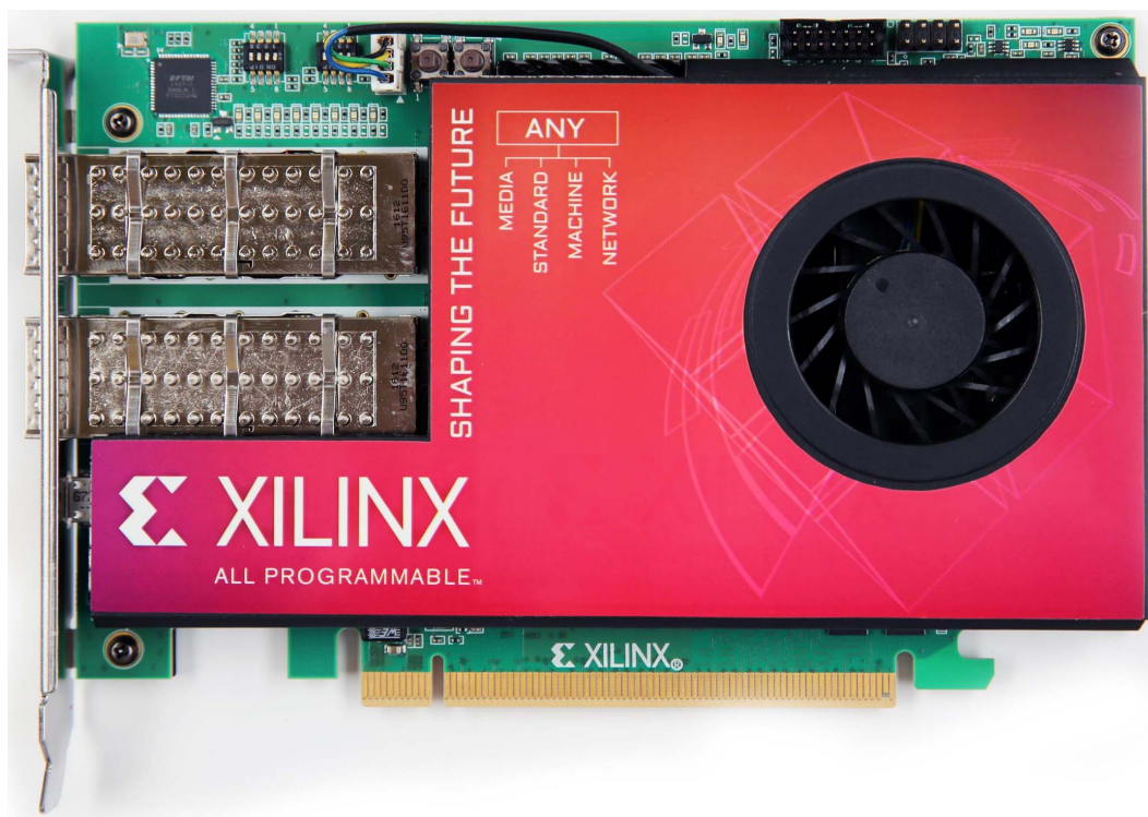
Figure 1-1: KCU1500 PCIe Data Center Board
