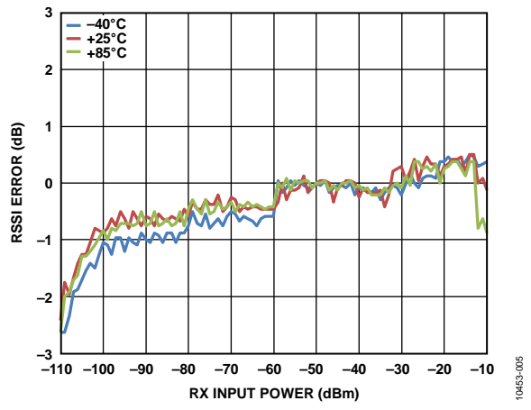
Figure 5. RSSI Error vs. RX Input Power, Edge Modulation (Referenced to -50 dBm Input Power at 800 MHz)
