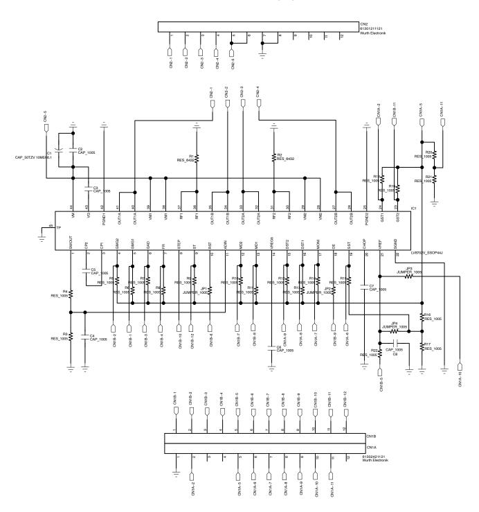
Figure 3. LV8702VSLDGEVB Schematic
