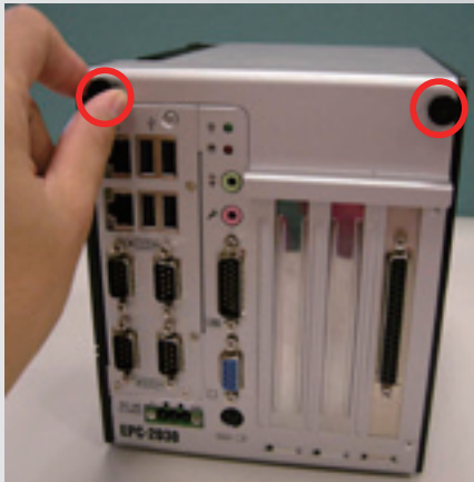
Thumbscrew Design for Easy, Tool-free Installation
