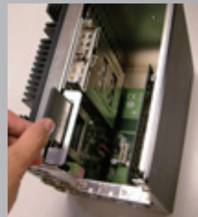
CFast Card Installation
