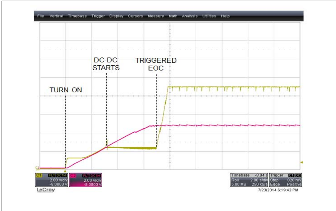
Figure 13. Buck-boost startup ( I_{IN} = 5\ \mu\text{A} )
