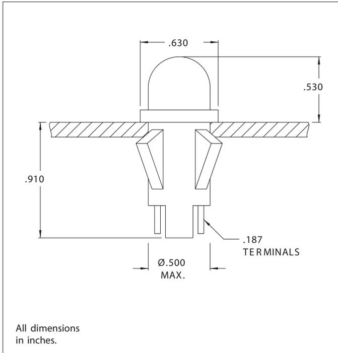
Mounting: Will snap-fit into Ø.500/.505 hole in panels .020/.100 thick. Push-on speednut SN0461 also available. Mounting hole pattern on page SP2.
