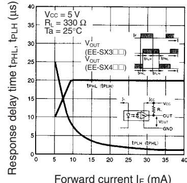
3. The following illustrations show the definition of response delay time. The value in the parentheses applies to the EE-SX401.
