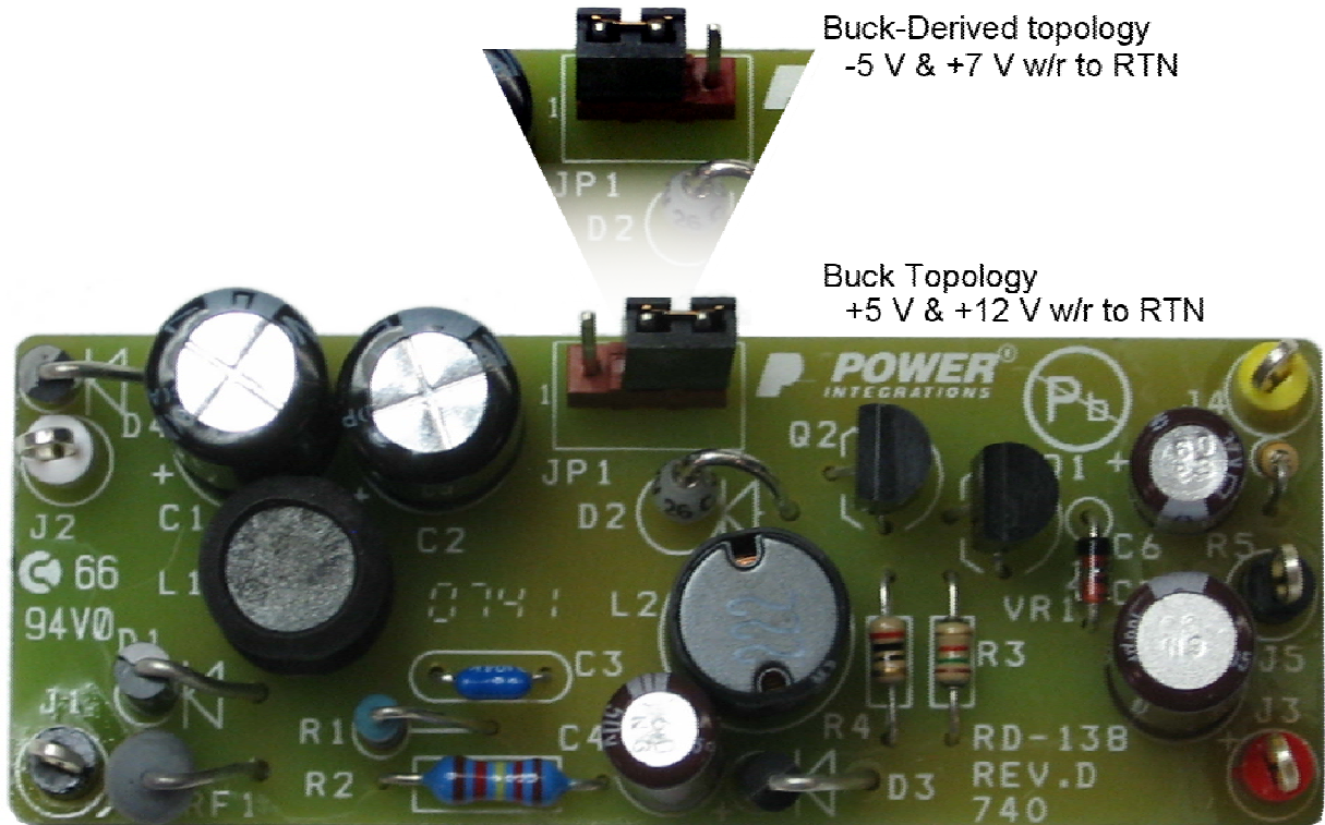
Figure 1 – Populated Circuit Board Photograph.
