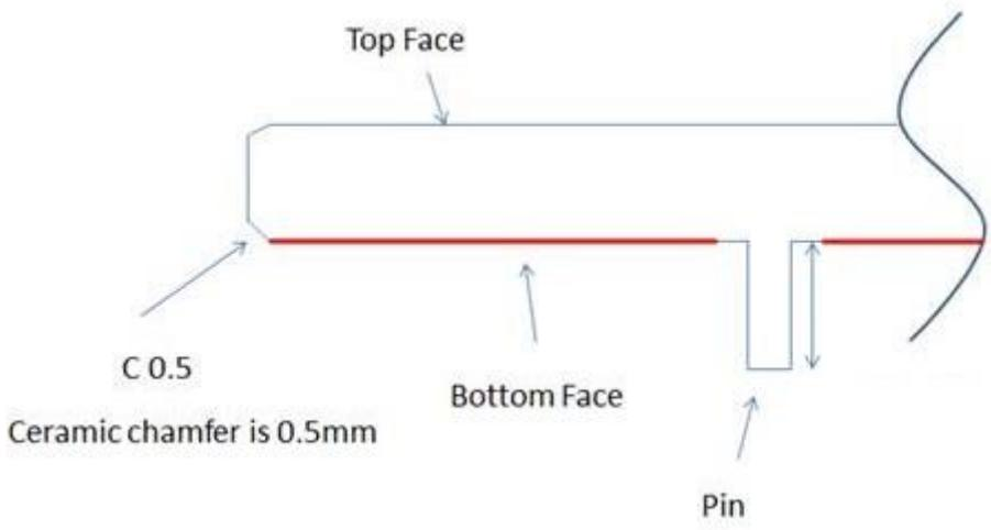
Red Line shows the adhesive without Liner – thickness 0.08~0.1mm
