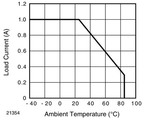
Fig. 2 - Allowable Load Current vs. Ambient Temperature
