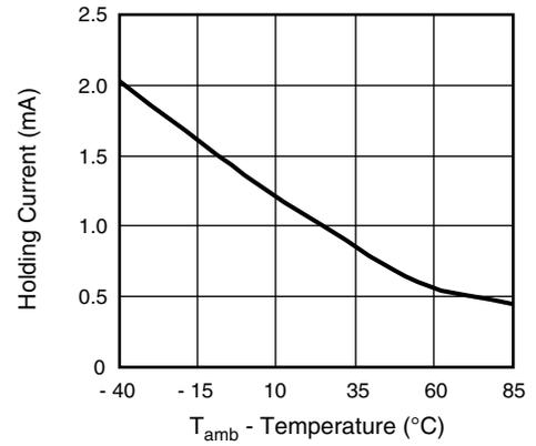
Fig. 10 - Normalized Holding Current vs. Temperature
