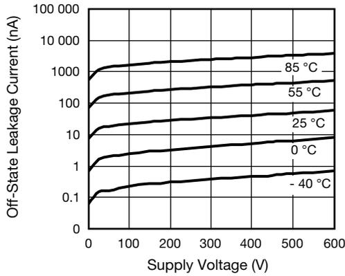
Fig. 7 - Off-State Leakage Current vs. Voltage
