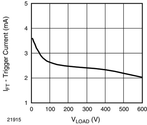
Fig. 12 - Trigger Current vs. V<sub>LOAD</sub>
