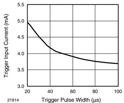
Fig. 11 - Trigger Current vs. Trigger Pulse Width
