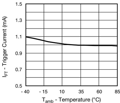
Fig. 8 - Normalized Trigger Input Current vs. Temperature
