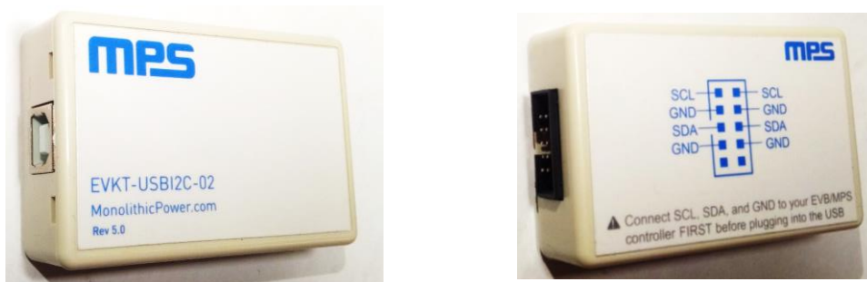
Figure 3: EVKT-USBI2C-02 Communication Interface
