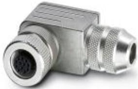
Connector, 12-position, shielded, Socket angled M12, A-coded, Solder connection, Knurl material: Zinc die-cast, nickel-plated, Cable gland Pg9, External cable diameter 6 mm ... 8 mm
