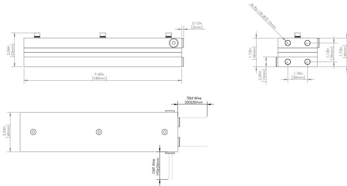
For overheating protection, the cooler is equipped with a bimetal thermostat. The maximum rating for the thermostat is 8 A. For systems with 8 A or less, the thermostat can be connected directly in series with the thermoelectric modules (TEMs). Otherwise, connect the TEMs to the power source through a relay of suitable rating which state is controlled with the bimetal thermostat.
