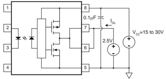
$I_{OL}$  Test Circuit
