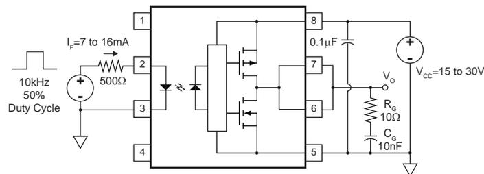
$t_{PLH}$ ,  $t_{PHL}$ ,  $t_r$ ,  $t_f$  Test Circuit
