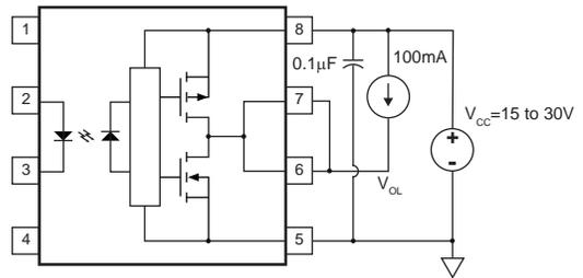
$V_{OL}$  Test Circuit
