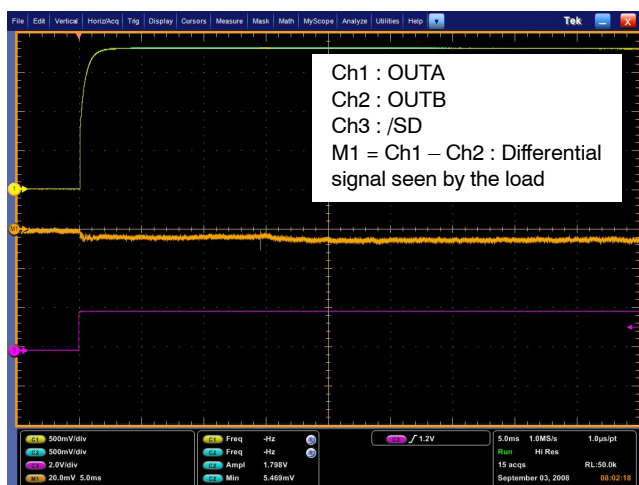
Figure 33. Zero pop noise turn on sequence with single-ended input to ground ( C_i = 47 \text{ nF} , R_i = 24 \text{ k}\Omega , R_f = 24 \text{ k}\Omega , C_{byp} = 1 \text{ }\mu\text{F} , R_l = 8 \text{ }\Omega , T_{on} = V_p )
