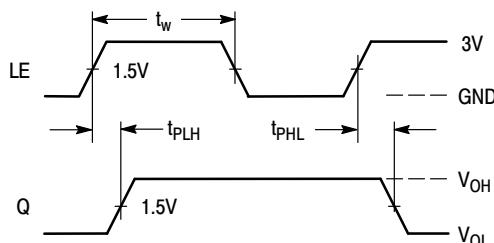
Figure 4. Switching Waveform
