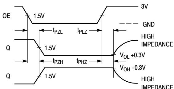
Figure 5. Switching Waveform
