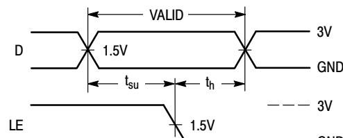
Figure 6. Switching Waveform
