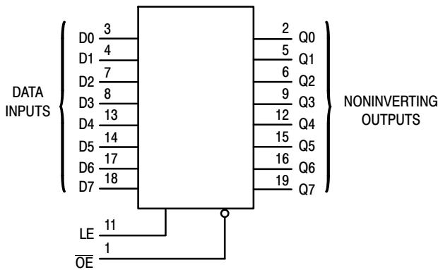
Figure 1. Logic Diagram
