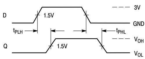
Figure 3. Switching Waveform
