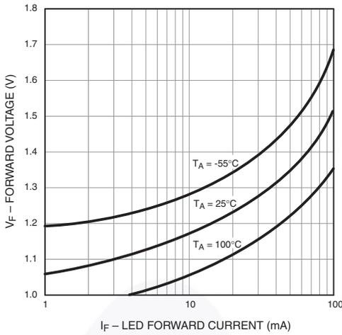
Figure 3. LED Forward Voltage vs. Forward Current
