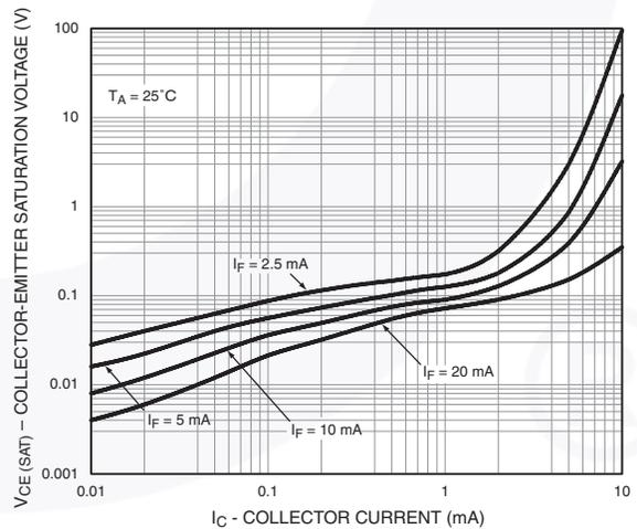
Figure 8. Collector-Emitter Saturation Voltage vs. Collector Current
