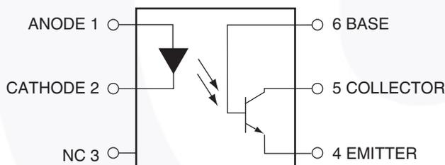
Figure 1. Schematic
