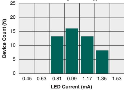
**Typical I<sub>F</sub> for Switch Dropout**
