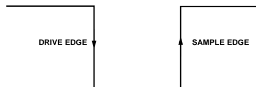
Figure 45. SPI Mode 3 SCLK Edges
