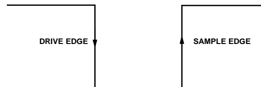
Figure 45. SPI Mode 3 SCLK Edges
