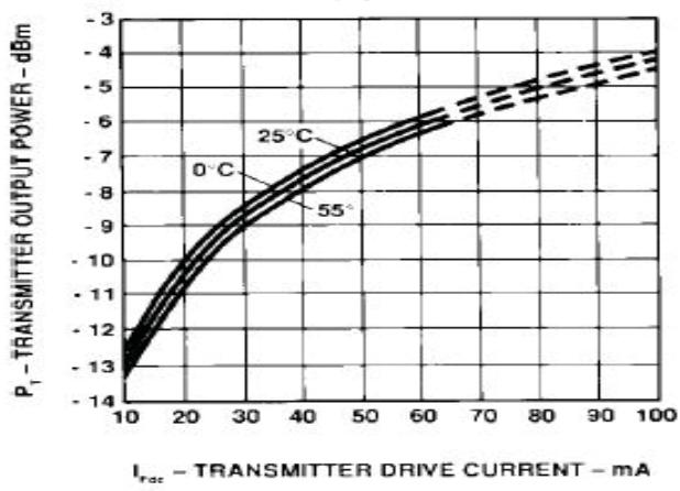
Figure 2. Typical transmitter output vs. forward current.
