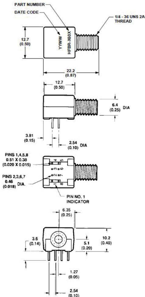
SMA is an industry standard fiber optic connector, available from many fiber optic connector suppliers. HFBR-4401Z is a kit consisting of 100 nuts and 100 washers for panel mounting the HFBR-0600Z components.
