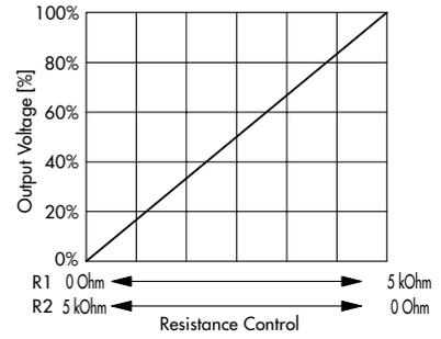
Connection for remote control voltage control
