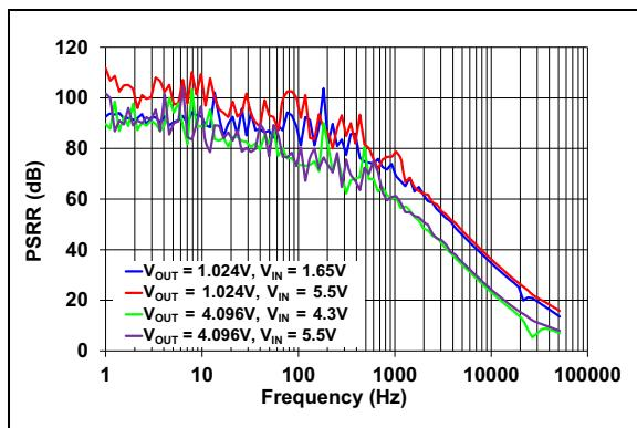
**FIGURE 2-14:** PSRR vs. Frequency, 1  $\text{k}\Omega$  Load,  $T_A = +25^\circ\text{C}$ .
