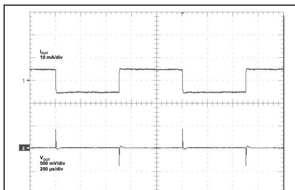
**FIGURE 2-24:** Load Transient,  $V_{DD} = 5.5$ ,  $V_{IN} = 2.5$ , 2.048V Option.
