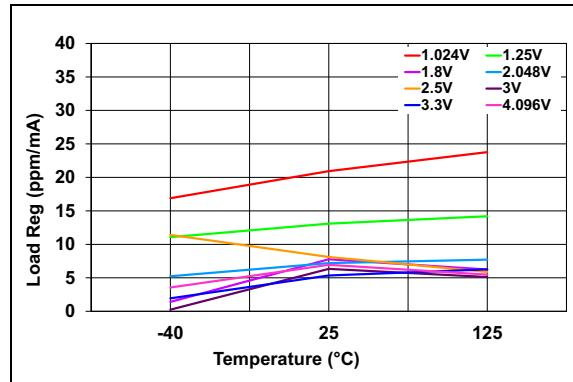
**FIGURE 2-4:** Load Regulation vs. Temperature,  $I_{LOAD}$  5mA Sink.
