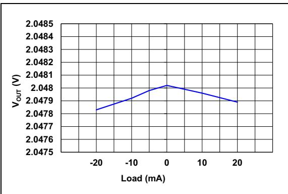
**FIGURE 2-19:**  $V_{OUT}$  vs. Load,  $T_A = +25^\circ\text{C}$ , 2.048V Option.
