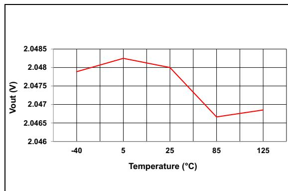
**FIGURE 2-2:**  $V_{OUT}$  vs. Temperature, No Load, 2.048V Option.
