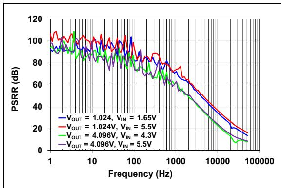
**FIGURE 2-13:** PSRR vs. Frequency, No Load,  $T_A = +25^\circ\text{C}$ .
