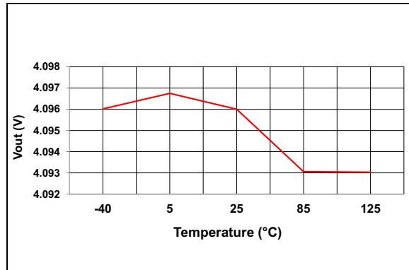
**FIGURE 2-1:**  $V_{OUT}$  vs. Temperature, No Load, 4.096V Option.
