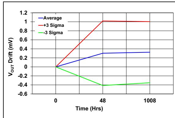
**FIGURE 2-18:**  $V_{OUPUT}$  Drift vs. Time,  $T_A = +25^\circ\text{C}$ , No Load, 800 Units.
