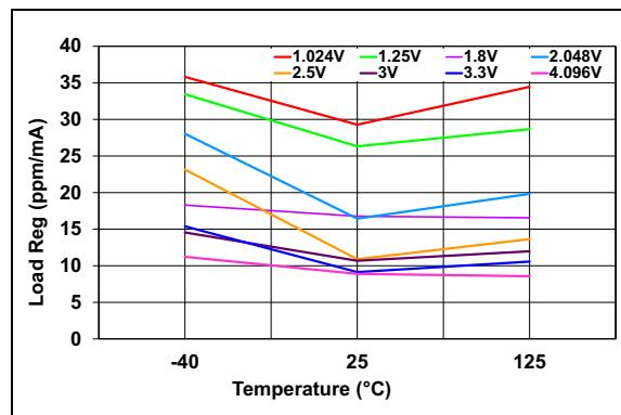
**FIGURE 2-5:** Load Regulation vs. Temperature,  $I_{LOAD}$  5mA Source.
