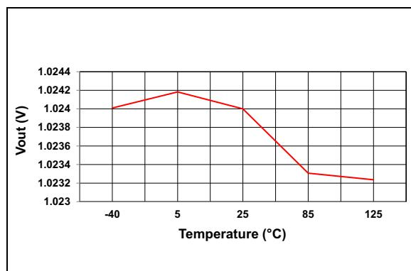
**FIGURE 2-3:**  $V_{OUT}$  vs. Temperature, No Load, 1.024V Option.
