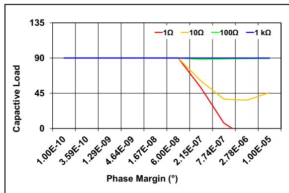
**FIGURE 2-26:**  $R_{ISO}$  vs.  $C_{LOAD}$ , 4.096V
