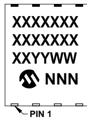
8-Lead DFN-S (6x5x0.9 mm)
