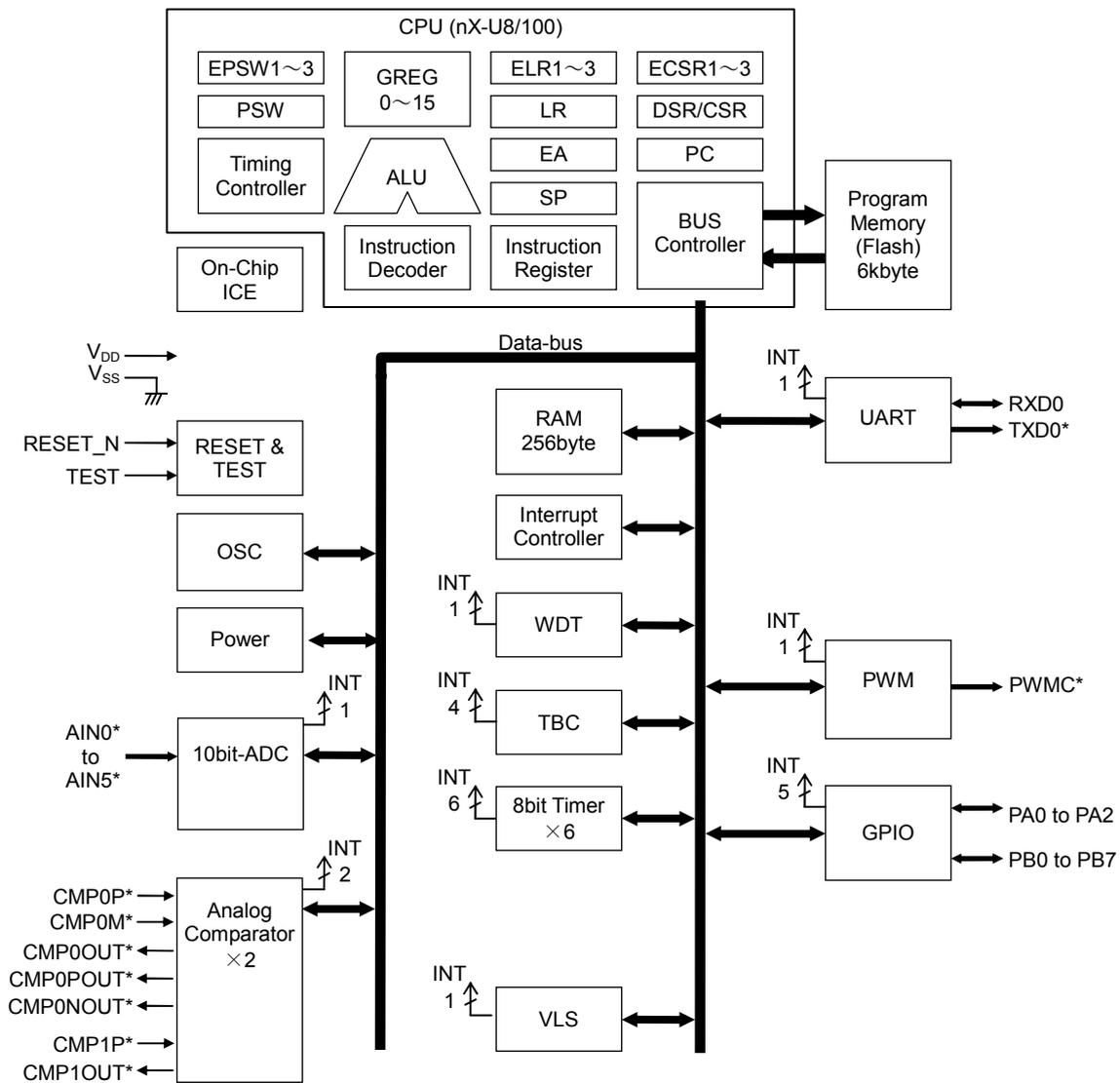
Figure 2 ML610Q102 Block Diagram
