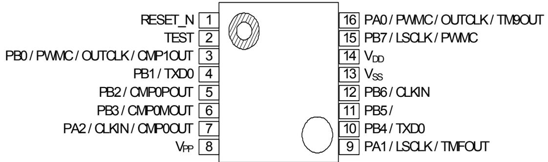
Figure 3 ML610Q101/ML610Q102 SSOP16 Pin Configuration
