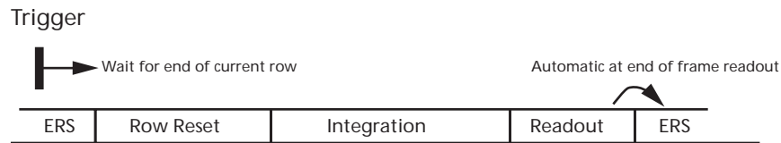
Figure 33: Entering and Leaving a Global Reset Sequence
