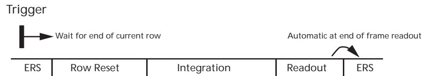
Figure 33: Entering and Leaving a Global Reset Sequence
