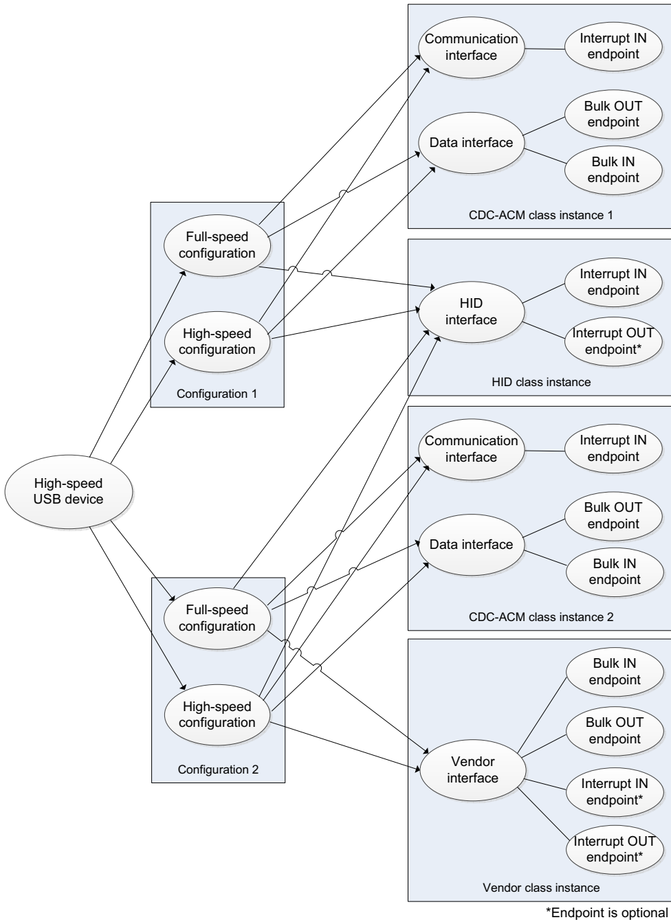
Figure 5-2 Complex Composite High-Speed USB Device Structure
