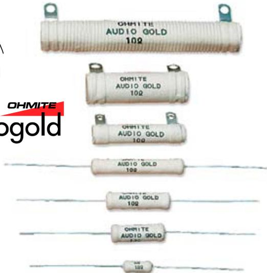
Ohmite now offers the Audio Gold Resistor Family, specifically designed for high-end loudspeaker and amplifier applications. These resistors utilize high quality resistance wire wound on a ceramic core, terminated, and finished with our flameproof Centohm® coating.
