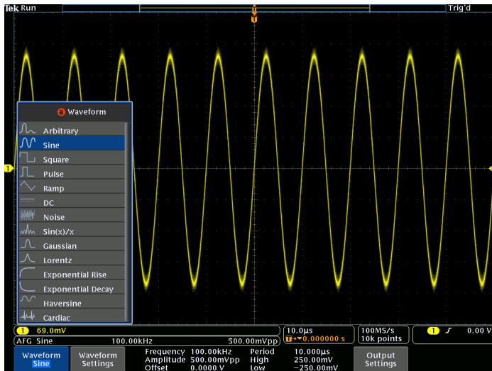
Waveform type selection in the integrated AFG.
