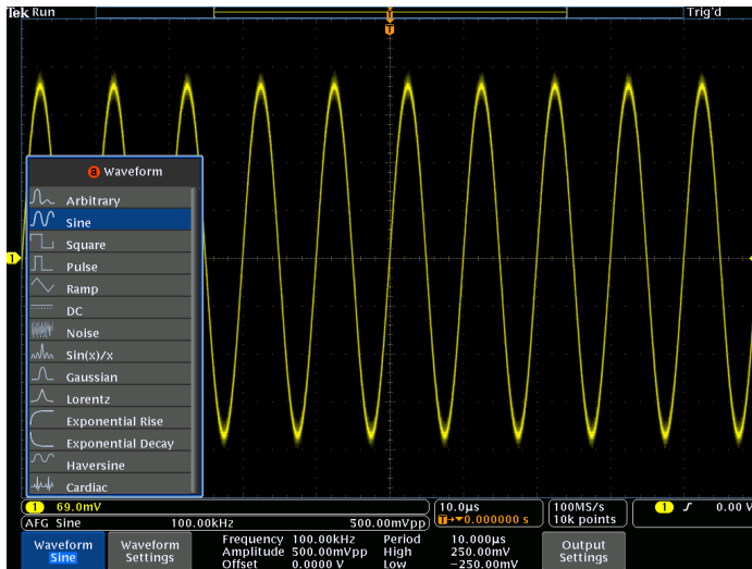
Waveform type selection in the integrated AFG.
