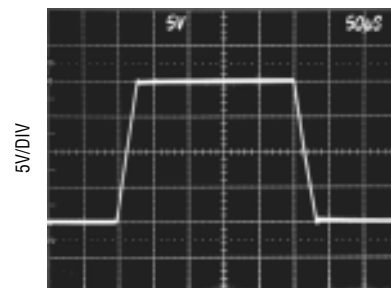
Large-Signal Transient Response
