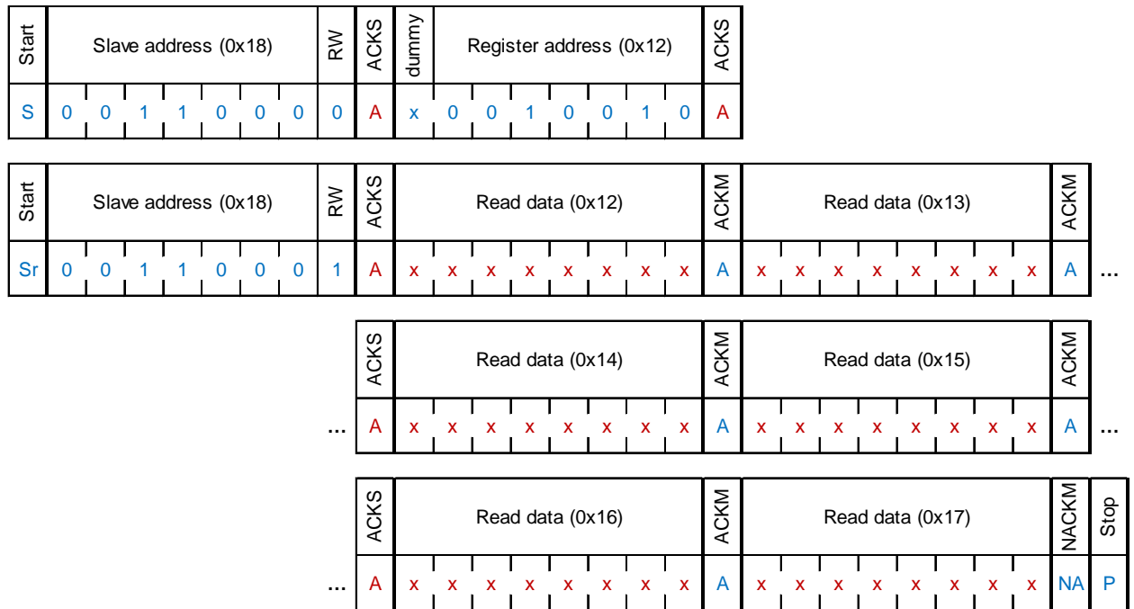
Figure 5: I 2 C multiple read
