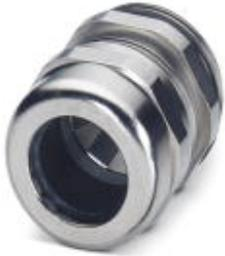
Cable gland, Cable gland material: Brass, nickel-plated, External cable diameter 9 mm ... 13 mm, Shielding: Yes, Connecting thread: M20, Color: silver
