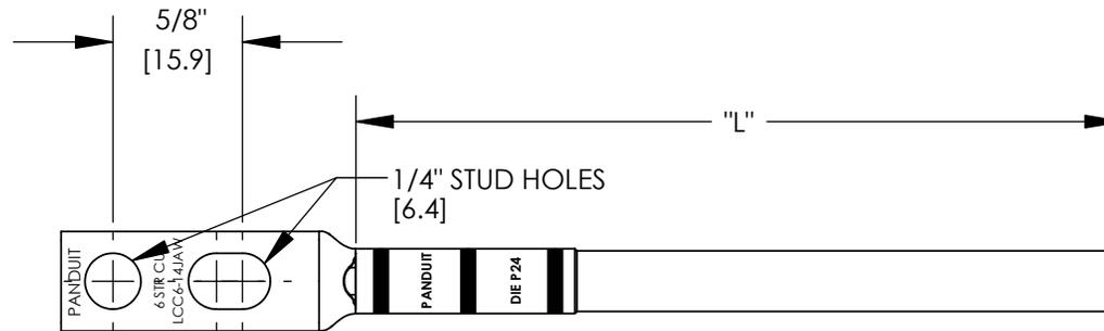
FACTORY CRIMPED #6 AWG/16mm SQ. JUMPER WIRE ASSEMBLY (QTY. 1) INCLUDES:
