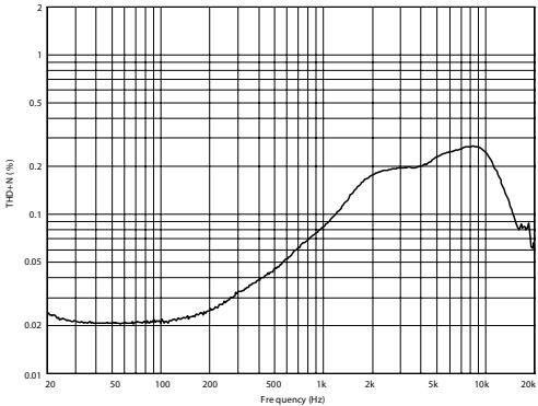
**Figure 14: THD vs. frequency (100 mW)**
