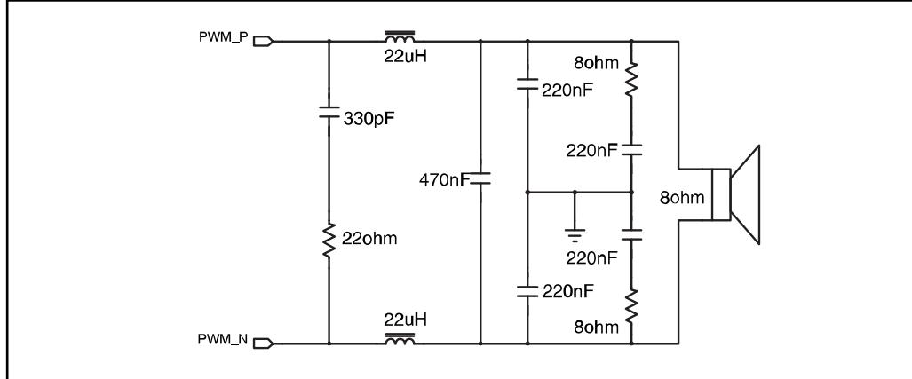
**Figure 24: Typical LC filter for a 6 Ω speaker**
