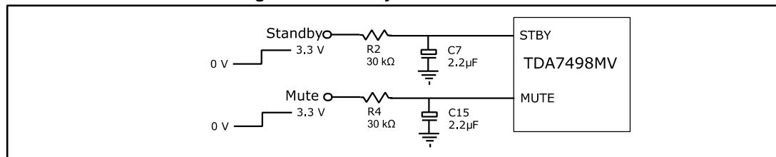
**Figure 20: Turn on/off sequence for minimizing speaker “pop”**
