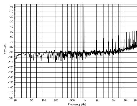
**Figure 17: FFT performance (-60 dB)**
