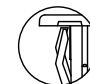
DETAIL VIEW VH1, VH3 & VH5 HOLE PLUGS (No wing serrations for ease of removal)
