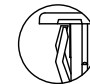
DETAIL VIEW VHP1, VHP3 & VHP5 HOLE PLUGS (No wing serrations for ease of removal)
