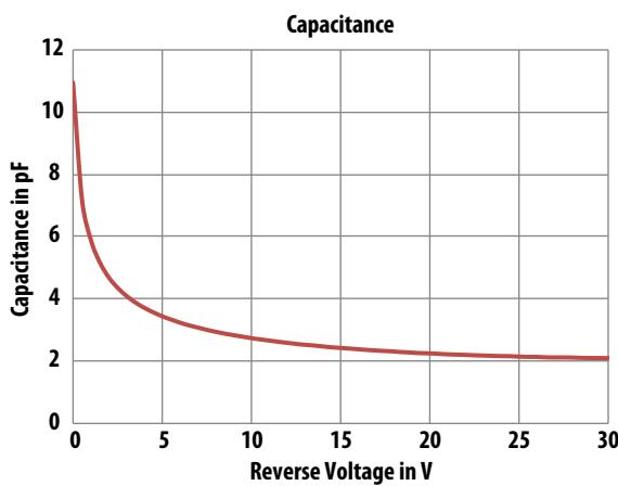
Figure 5. Typical Capacitance; measured at  $TA=25^\circ C$  with  $f_{measured} = 1MHz$
