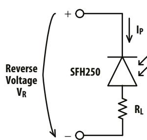
Figure 4 .Test circuit
