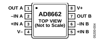
Figure 4. AD8662, 8-Lead MSOP (RM-8)
