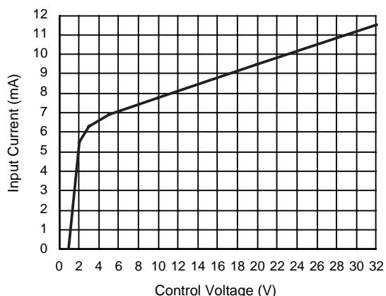
Figure 2 — Control Characteristic
