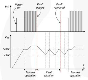
Figure 19. Auto-Restart Protection Waveforms
