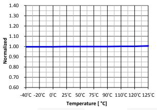
Figure 11. UVLO Threshold Voltage (V<sub>START</sub>) vs. T<sub>A</sub>
