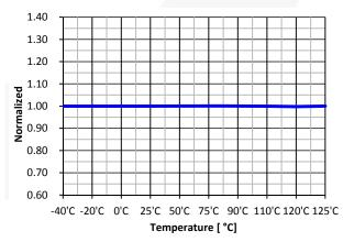
Figure 16. Maximum Duty Ratio (D<sub>MAX</sub>) vs. T<sub>A</sub>
