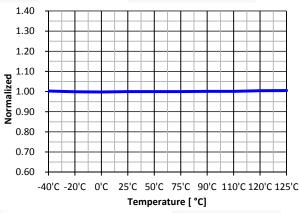
Figure 14. Over-Voltage Protection (V<sub>OVP</sub>) vs. T<sub>A</sub>
