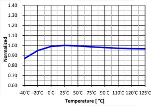
Figure 7. Startup Charging Current (I<sub>CH</sub>) vs. T<sub>A</sub>
