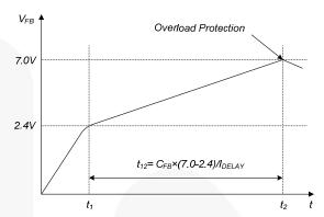
Figure 20. Overload Protection
