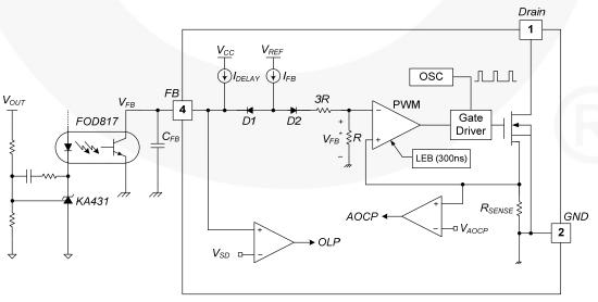
Figure 18. Pulse Width Modulation Circuit
