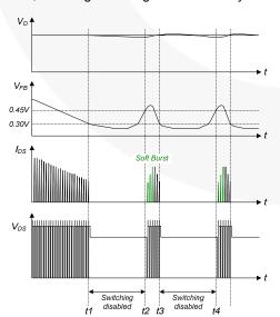
Figure 22. Burst-Mode Operation
