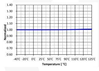
Figure 13. Shutdown Feedback Voltage ( $V_{SD}$ ) vs.  $T_A$
