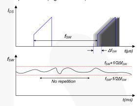
Figure 23. Random Frequency Fluctuation
