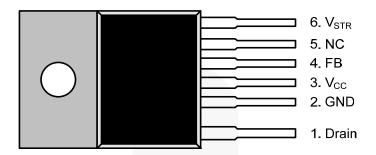
Figure 3. Pin Configuration (Top View)
