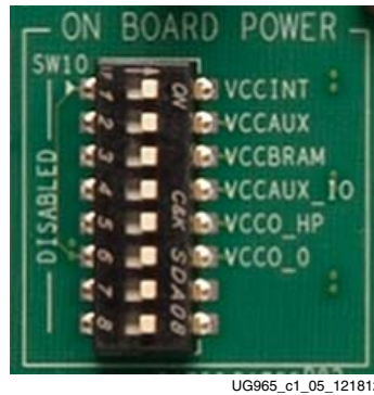
Figure 1-5: Core Power Regulator Enable Switches SW10
